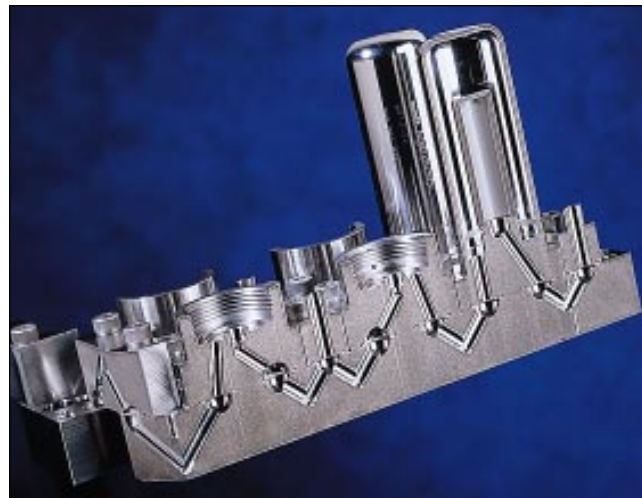
Figure 2. Cross section through a Z-Bloc system shows the “V”-shaped passages through the substrate that connect the top-mounted components. A jumper between substrates is shown on the left.
