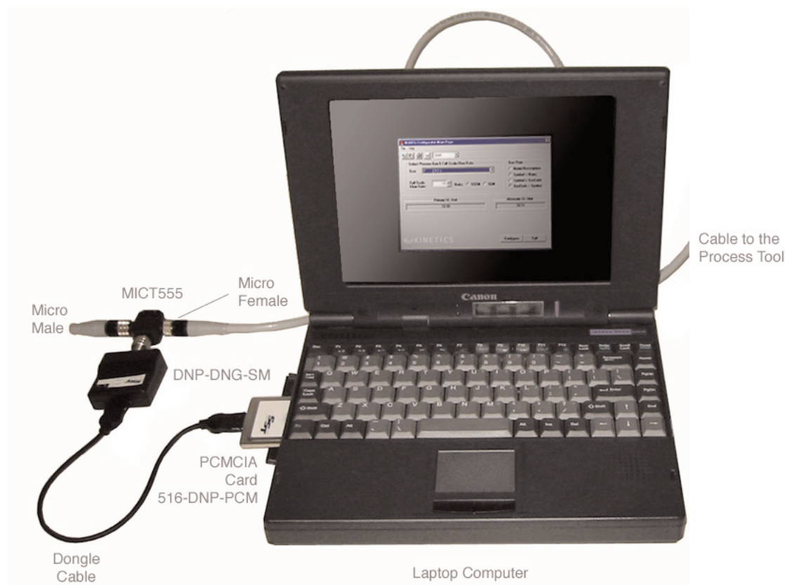
Figure 6.1 Typical connection for a DeviceNet MFC to the MultiFlo Configurator bench set up
