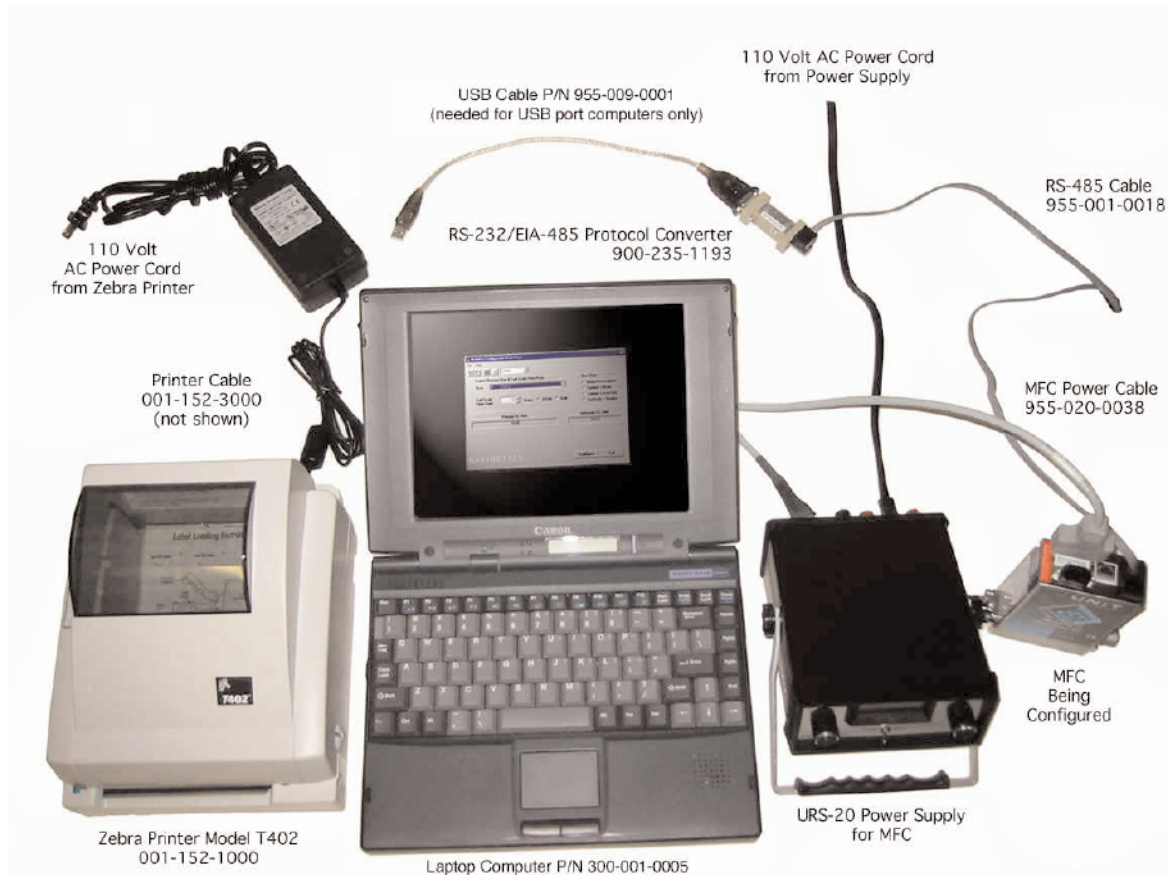
Figure 1.1 MultiFlo Configurator accessory kit p/n 535-400-2002
