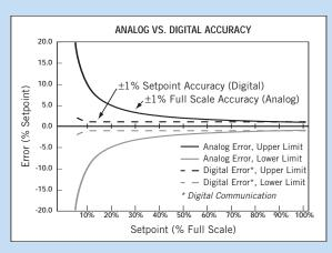
Digital model 8261 products have an accuracy of  $\pm 1\%$  of setpoint, while the analog model 8260 has an accuracy of ±1% full scale. (Accuracy chart reflects primary standard calibration.)
